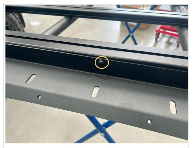
13. Fit the Front panel to the rack assembly. Secure to the pre-placed nuts in the front extrusion using the M8x12 Button head bolts and flat washers.
