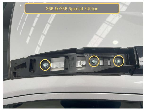
36. Using a 10mm Socket, remove the 3x bolts securing the front mount of the roof rail to the captive nuts in the roof.
