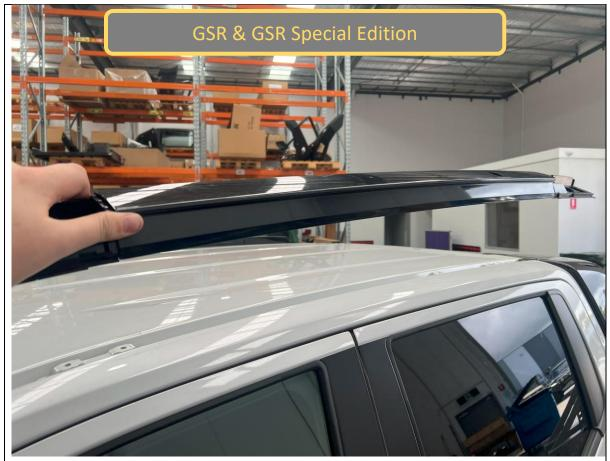
38. The roof rail should now be loose. Carefully lift the roof rail away from the car and set aside.
