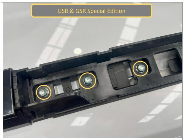
37. Using a 10mm Socket, remove the 3x bolts securing the rear mount of the roof rail to the captive nuts in the roof.
