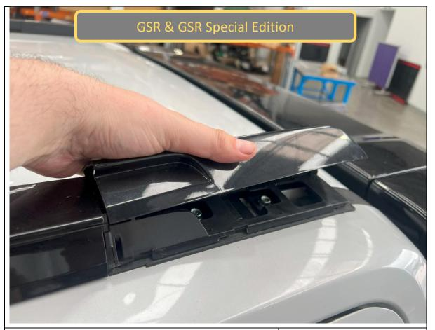
33. Using a trim tool, carefully pry up the rear roof rail cover, using similar technique to the front cover.
