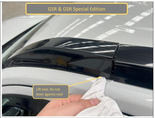
32. Using a trim tool, carefully pry up the front roof rail cover. There are molded clips in the cover securing it to the roof rail.
